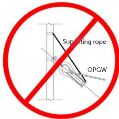
Improperly supported sheave
