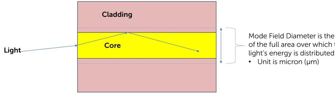
Mode Field Diameter is the width of the full area over which the
