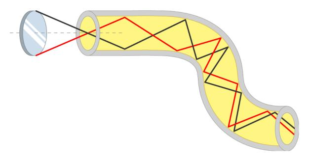
Light constantly bounces from the cladding back into the core as it travels down the fiber
