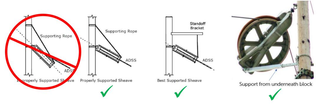
The ADSS and the block must be in the same plane during the pull!
