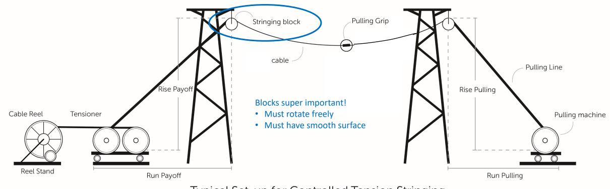
Typical Set-up for Controlled Tension Stringing
