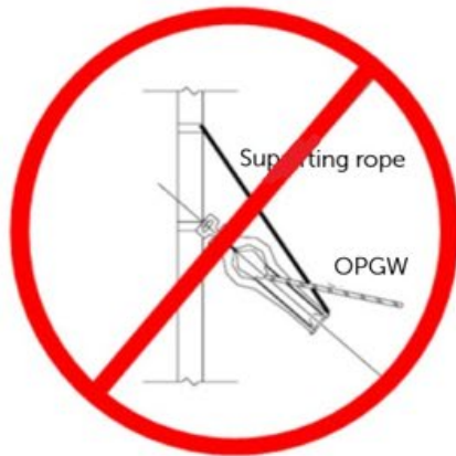
Improperly supported sheave
