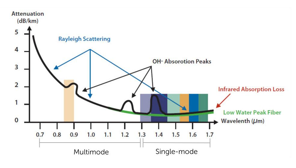
Fiber attenuation as a function of wavelength
