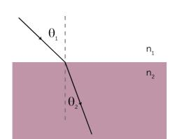
n<sub>1</sub>: index of refraction of medium 1 n<sub>2</sub>: index of refraction of medium 2
