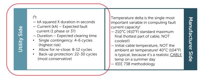
*And*, ready to move on to understand what data we need to calculate the required fault current capacity
