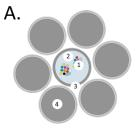
OPGW C Low CONSTRUCTION: 1. Optical fiber Corning SMF-28 Ultra 2. Water-blocking gel 3. Stainless Steel Loose Tube (SSLT) 4. Aluminum-Clad Steel Wire (ACS)
